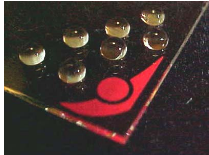
100° average contact angle (goniometer)
